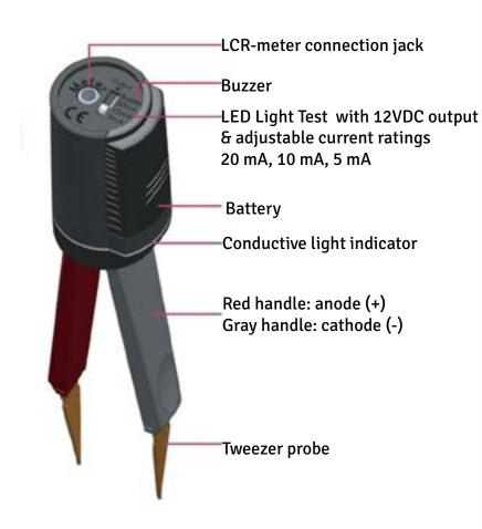
**Warning: Do Not Test Electrified Components**
